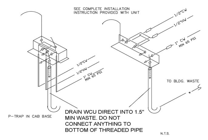
DO NOT CUT FACTORY SUPPLIED THREADED BRASS PIPE - VOIDS WARRANTY. SLEEVE FACTORY PIPE INTO 11/2" BUILDING WASTE
