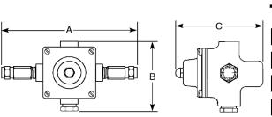
Thermostatic Mixing Valve Model 911®E/F Emergency Ev ENG. NO. 84907-D PAT. NO. 5,011,074. PAT. NO. 5,379,936.
