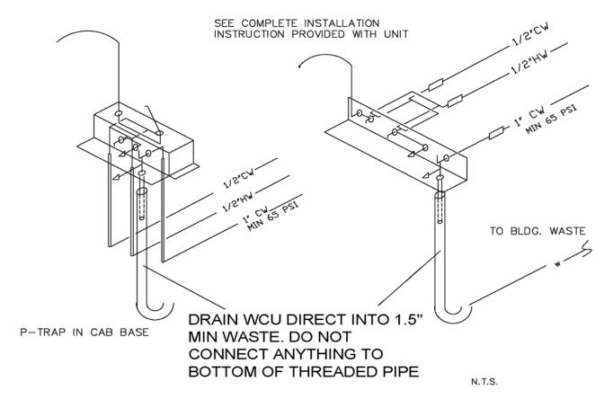
DO NOT CUT FACTORY SUPPLIED THREADED BRASS PIPE - VOIDS WARRANTY. SLEEVE FACTORY PIPE INTO 1½" BUILDING WASTE
