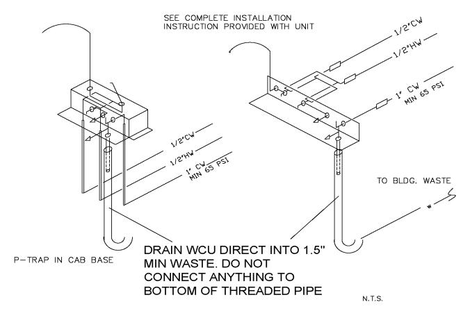
DO NOT CUT FACTORY SUPPLIED THREADED BRASS PIPE - VOIDS WARRANTY. SLEEVE FACTORY PIPE INTO 12" BUILDING WASTE
