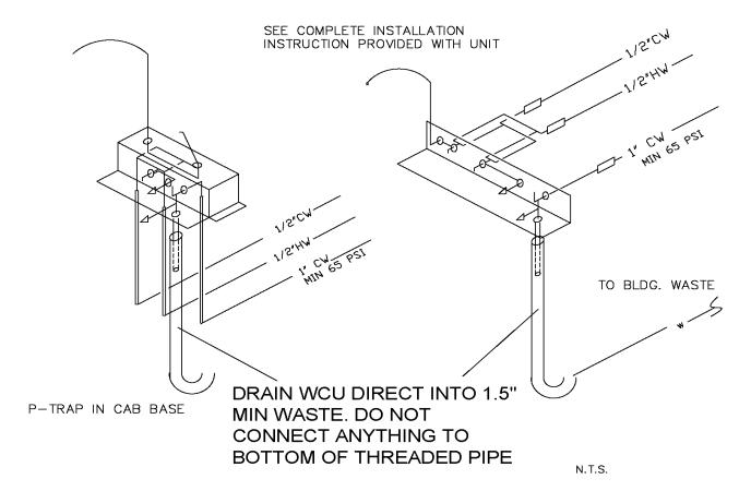
DO NOT CUT FACTORY SUPPLIED THREADED BRASS PIPE — VOIDS WARRANTY. SLEEVE FACTORY PIPE INTO  $1\frac{1}{2}$ " BUILDING WASTE
